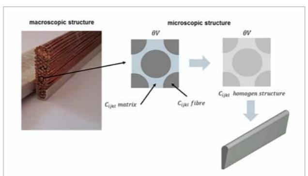
Fig. 2: Homogenization
