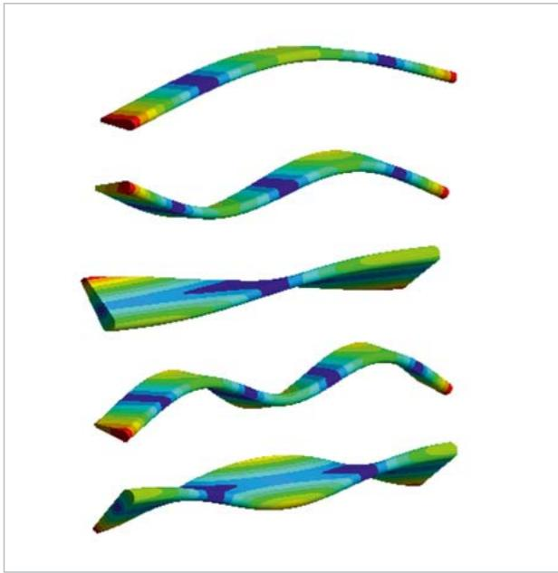
Fig. 3: Mode shapes of the slot bar | top down - 1st bending, 2nd bending, 1st torsion, 3rd bending, 2nd torsion
