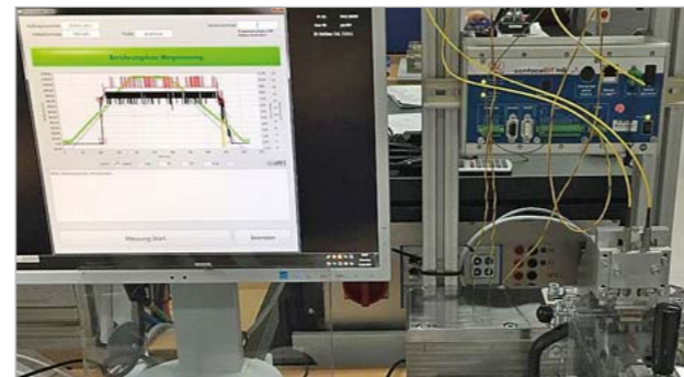
Fig 6: Measurement of mechanical characteristics under laboratory conditions on an open relay
