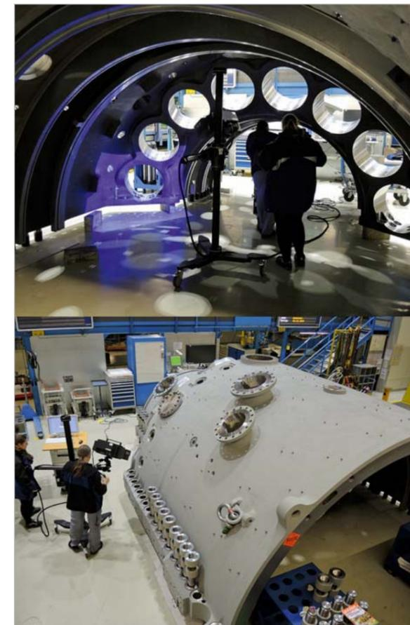
Fig. 1: Measurement of true geometry using laser scans
