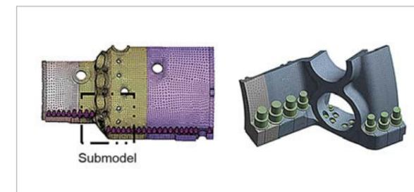
Fig. 7: Submodel of turbine housing
