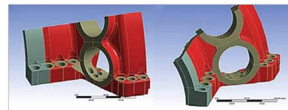
Fig. 6: Red: Surface parts to be varied, Gray: machined surface parts (fixed)
