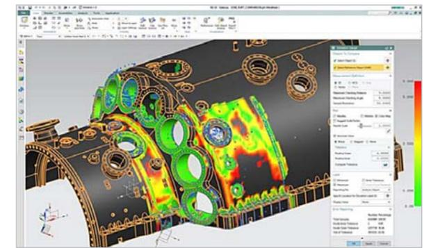
Fig.2: Post processing of laser scan data in SIEMENS NX
