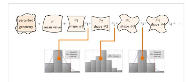
Fig. 3: Statistical shape model (Random field) to include geometric scatter in SoS
