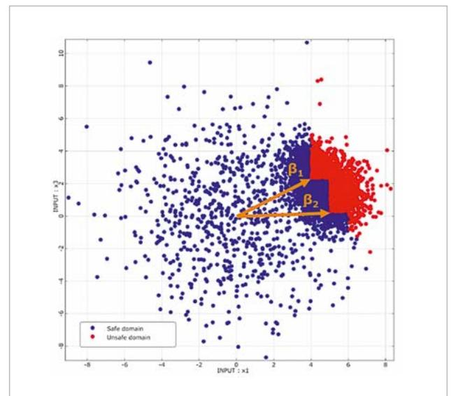
Fig. 3: Adaptive Importance Sampling for a linear limit state function considering discrete random variables, samples in the standard Gaussian space.
