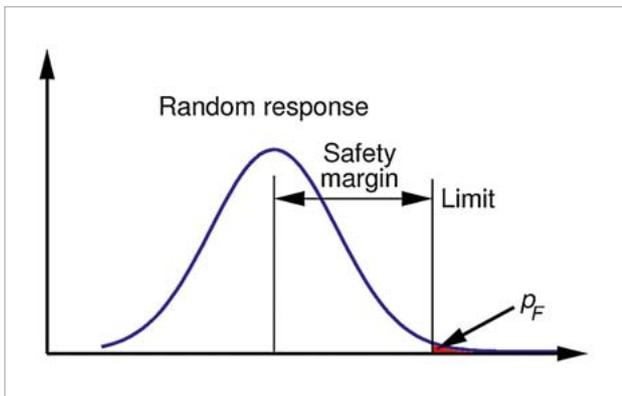
Fig.2: Scatter of a fluctuating response with safety margin (distance between mean and the failure limit) and the corresponding probability of failure  $p_F$ .
