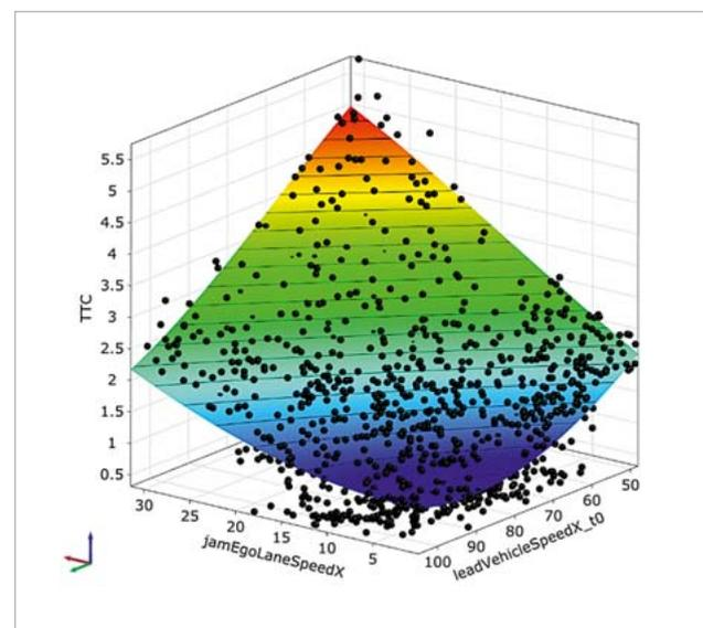
Fig. 5: Jam end scenario: adaptive meta-model used for the verification of the reliability algorithms
