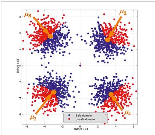
Fig. 4: Importance Sampling using Design Points generated by a multi-modal sampling density which consists of several standard normal densities.
