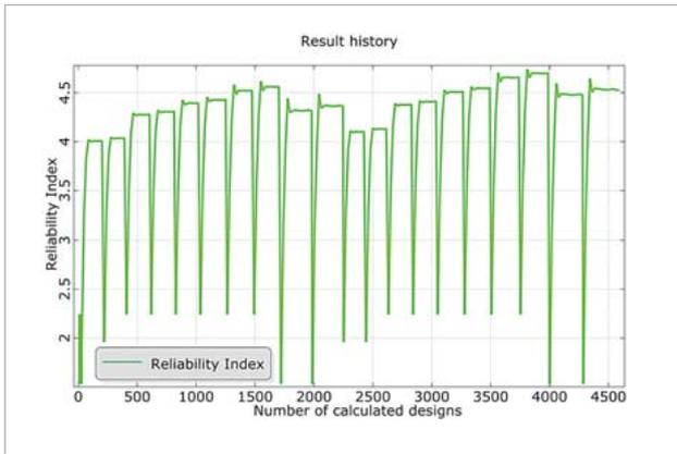
Fig. 6: Convergence of the multi FORM-search assuming a limit of 0.5s for the time-to-collision
