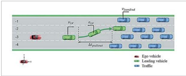
Fig. 1: Jam end traffic scenario on the highway. By altering the input parameters this logical scenario can be varied in its characteristics.
