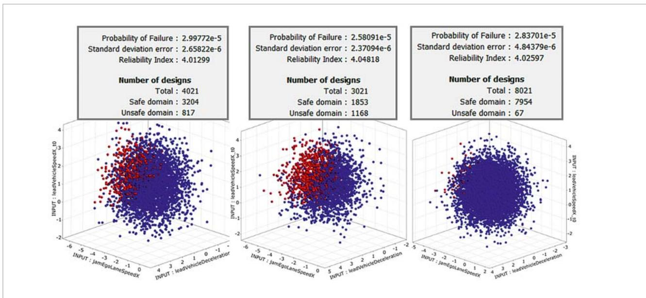
Fig. 8: Influence of the accuracy of the obtained most probable failure points using a limit of 0.5s on the meta-model: left – original results, middle – failure points are located in unsafe region, right – failure points are located in safe region
