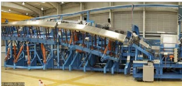
Fig. 2: Test rig of the A380. In the front, drive systems and load cylinders to simulate the air load.
