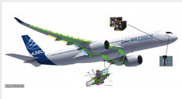
Fig. 1: Principle structure of the High-Lift System (HLS)
