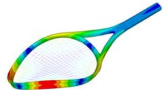
Torsion mode of a tennis racquet illustrating how a non-center hit introduces torsion.
