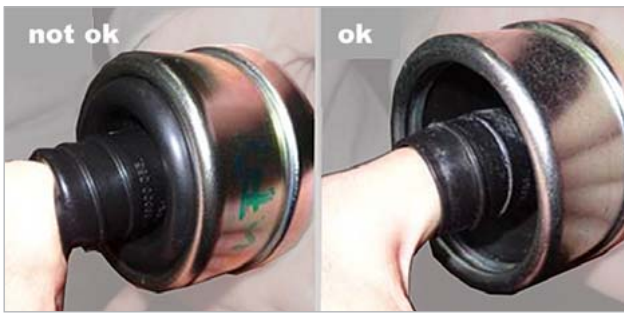
Fig. 2: "S-punch shaped" deformation (left) and optimal rolling off behavior (right) of the rubber boot
