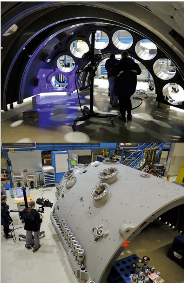
Fig. 1: Measurement of true geometry using laser scans
