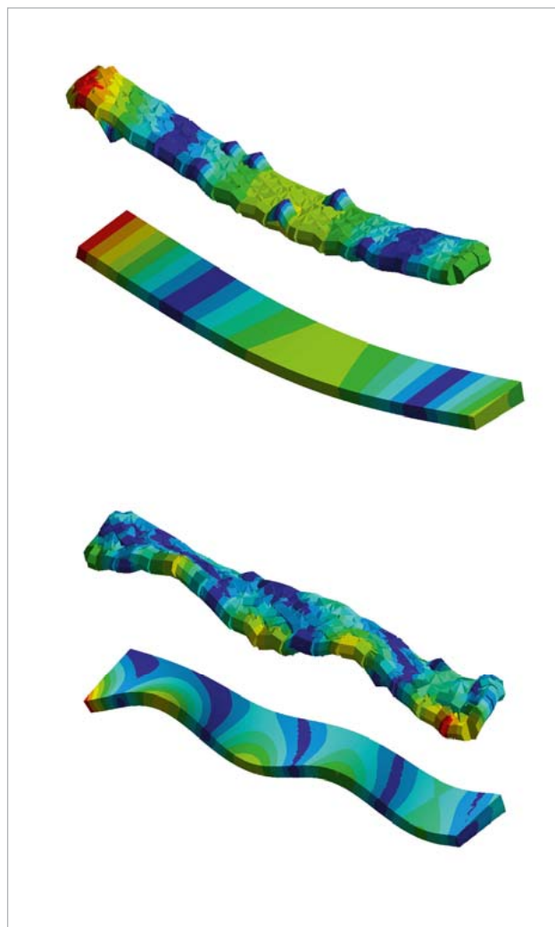
Fig. 3: Comparison of the experimental (top) and simulated mode shapes
