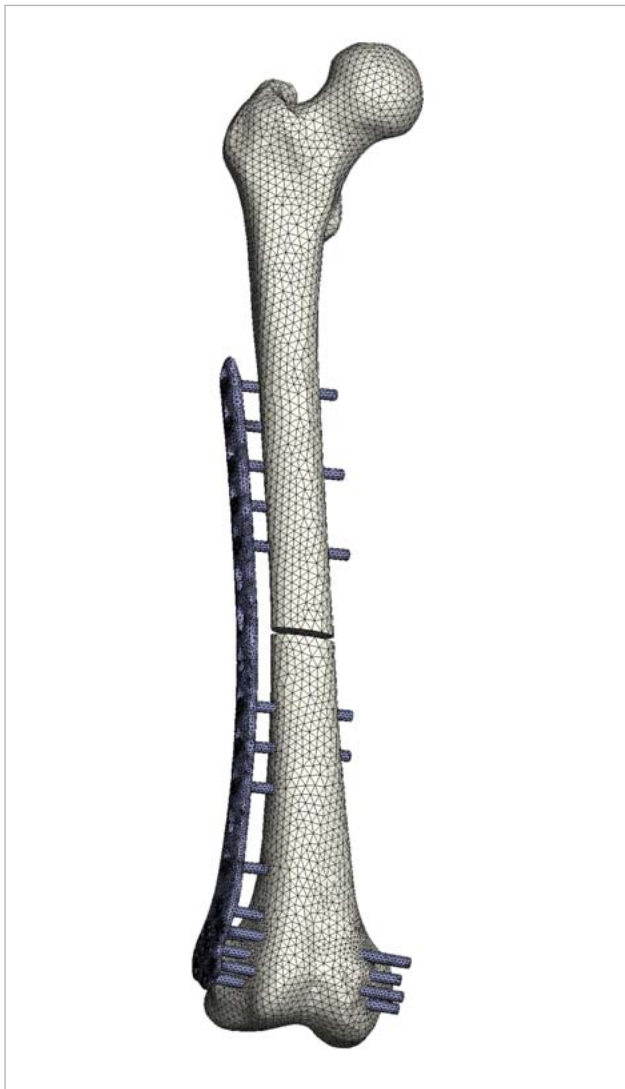
Fig. 5: Meshed bone with plate and screws
