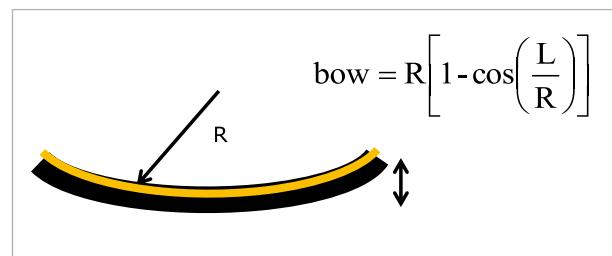
Fig. 2: Curvature radius a Cu-Si bimetallic strip is the raw measured quantity. The bow is calculated afterwards and compared with simulation results.
