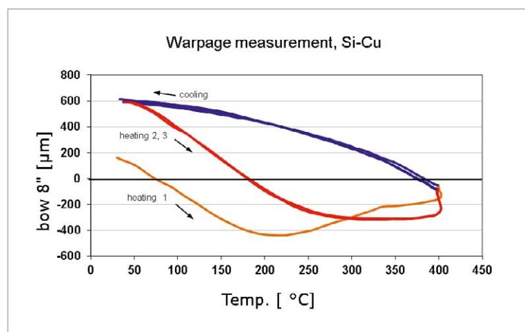
Fig. 4: Bow evolution displayed as a function of temperature clearly demonstrates complex the inelastic behavior of ECD copper.
