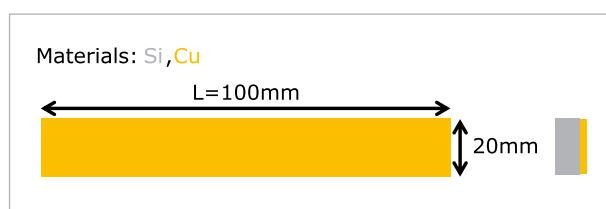
Fig.1: Bimetallic strip in top view and cross section, silicon in grey, copper in yellow
