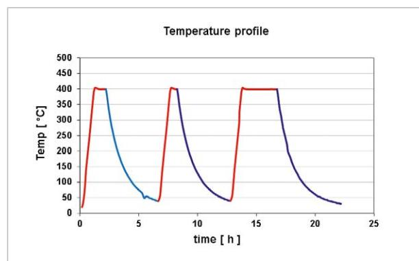
Fig. 3: A typical cyclical heating and cooling process during a measurement of a Cu-Si bimetallic strip
