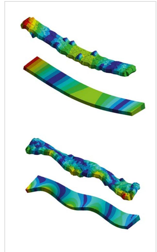
Fig. 3: Comparison of the experimental (top) and simulated mode shapes
