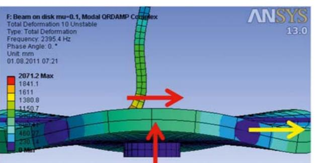
Figure 2: Brake disk picks up brake pad
