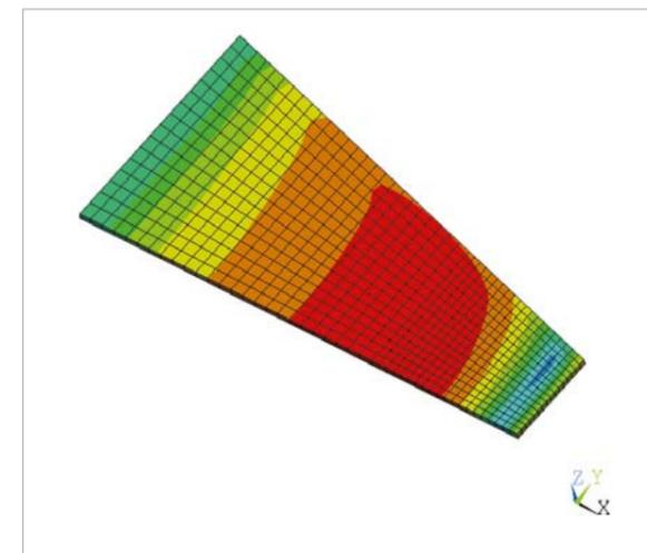
Fig. 5: Shear stress distribution in the interface layer
